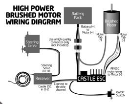
connect to the red wire (or positive + side hood) on your motor, and the black wire to the black wire (or negative - side hood) of the motor. The white motor wire (or center connector on the ESC) is not used. After calibration, (explained later) you may need to swap the two motor wires to get the wheels to spin in the right direction.
